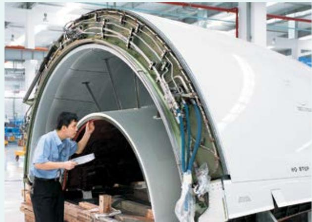
Based at Jinjiang in Fujian Province in Mainland China, HAECO Spirit AeroSystems specialises in aerostructure repair and overhaul services.
