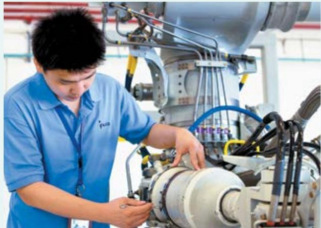
Based in Xiamen in Mainland China, HAECO Landing Gear Services completed its first repair and overhaul of Boeing 747-8 landing gear in 2017.
